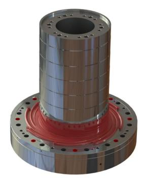
The spiral distribution zone, located between the second and third plates, is designed to provide improved mixing, thermal consistency and polymer dispersion. The polymer flows across the spiral distribution zone toward the central pin. The polymer reaches the central pin and turns 90 degrees upward to the next layer or die lip. The central pin has internal heaters to assistance in start-up and preserve process control.
